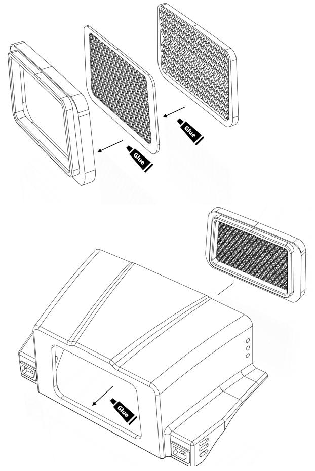
Installing the lights M2x5mm x4  $\bigcirc$  $\bigcirc$ Orange 3mm White 3mm LED x2 LED x2  $\bigcirc$  $\bigcirc$  $\bigcirc$ 00 0 0 0 0 **Repeat on the** 0 other fender cover Ī
